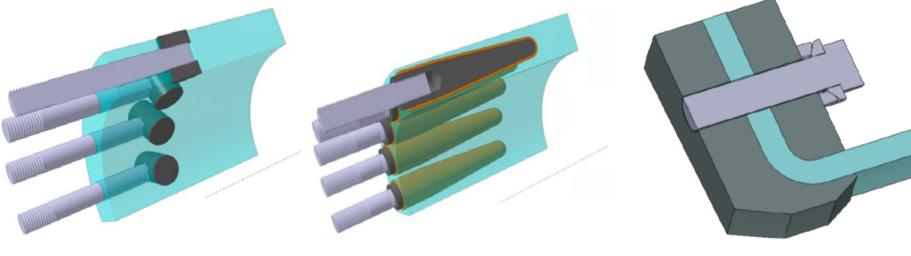
Common root connectors<sup>[1]</sup> : T-Bolts / Bonded inserts
