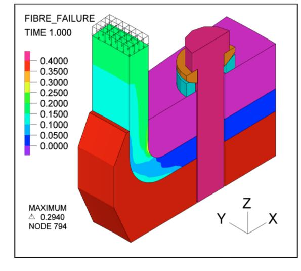
Puck Fibre Failure exposition factor
